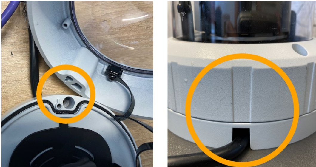
Figure 14: Top Cover Alignment
